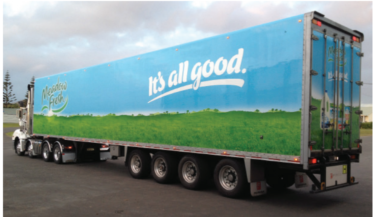
Goodman Fielder truck with red conspicuity tape outline. As you can see, it has minimal impact on your vehicle's daytime aesthetic, however it will have a huge impact on your vehicle's visibility at night.
