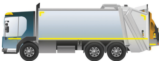
Rubbish truck with partial contour markings Many rubbish trucks will not be able to take a full line or contour marking due to the equipment being fitted. In these cases, it is acceptable to retain rear marker plates with conspicuity markings fitted to the fullest extent practicable.
