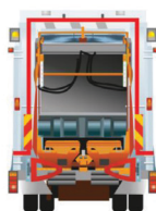
Rubbish truck with partial contour markings Many rubbish trucks will not be able to take a full line or contour marking due to the equipment being fitted. In these cases, it is acceptable to retain rear marker plates with conspicuity markings fitted to the fullest extent practicable.
